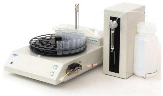
The tray configuration (number of positions, volumes of the vials) is variable. (standard: 89 x 8/4/2 ml, 53 x 16 ml, 36 x 30 ml, 18 x 50 ml), external positions (e.g. standards, control samples) are also possible. Two different kinds of trays are recognized automatically.
