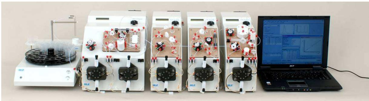
The **FIASampler** autosampler can accommodate two different sample trays with differing sample volumes. Its integrated dilutor prepares automated dilutions from off-range samples (degree of dilution variable).
