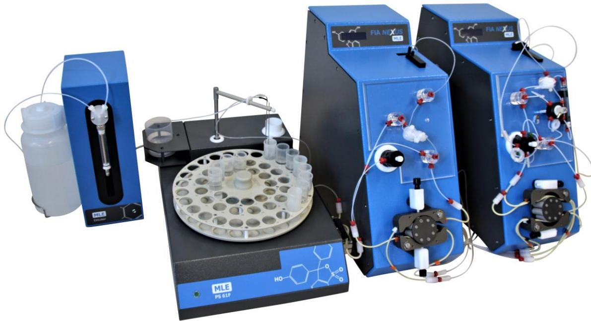
The autosampler **FIAsampler** can accommodate two different sample trays with differing sample volumes. Its integrated dilutor prepares automated dilutions from off-range samples (degree of dilution variable).
